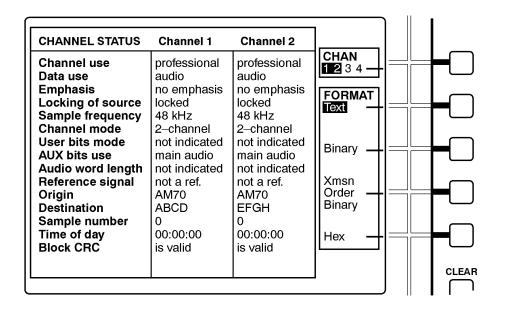
Figure 28: The Channel Status view, text mode
